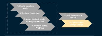
6. OPTIMIZATION AND DESIGN CHANGES Optimization and design changes are managed by refining the system and the degraded models, or by reviewing the fault model
