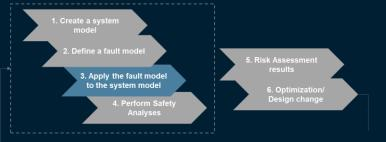
3. APPLY THE FAULT MODEL TO THE SYSTEM MODEL The fault model is automatically injected into the system model to to create a new extended model that foresee a degraded behaviour and understand the possible hazard
